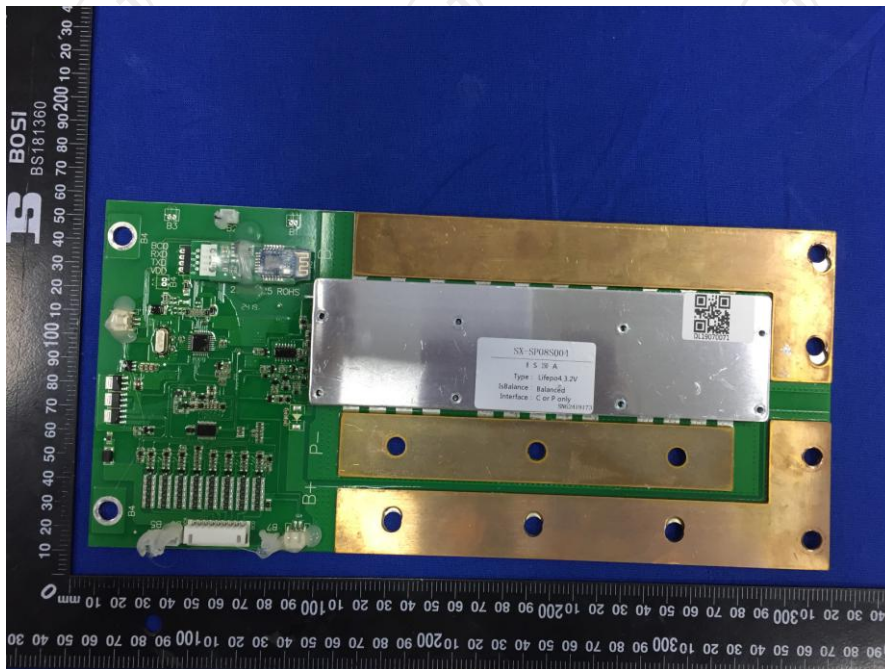
Picture 5. Protection board view
